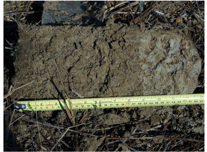
Figure 4. —The lower portion of this soil profile meets the color and depth requirements of indicator F3 (Depleted Matrix); however, the upper portion of the profile contains a layer with chroma of 2 or more that is more than 15 cm (6 inches) thick. As a result, indicator F3 (Depleted Matrix) is not met.
