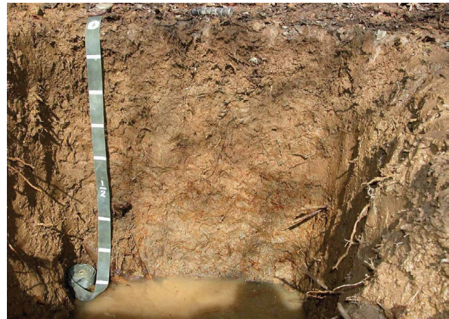
Figure 38.—Indicator F19 (Piedmont Flood Plain Soils). This indicator is restricted to active flood plains. It does not require a matrix color with chroma of 2 or less.
