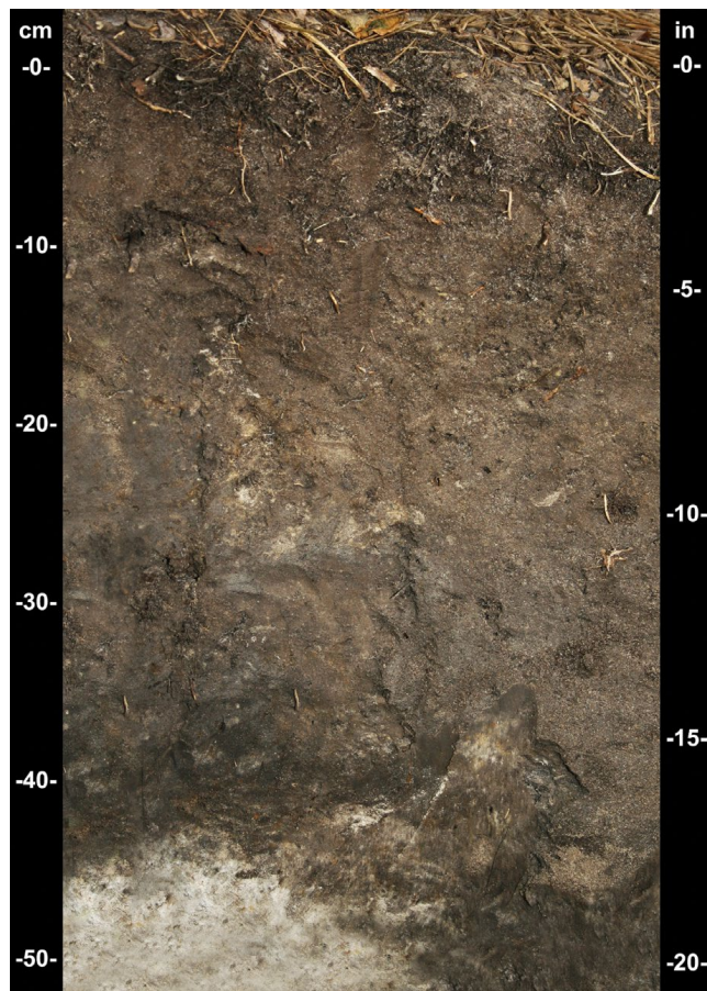
Figure 31.—Indicators F6 (Redox Dark Surface) and F7 (Depleted Dark Surface). A soil that meets the requirements of indicator F7 commonly also meets the requirements of indicator F6. If the dark surface layer has depletions, it most likely also has concentrations.
