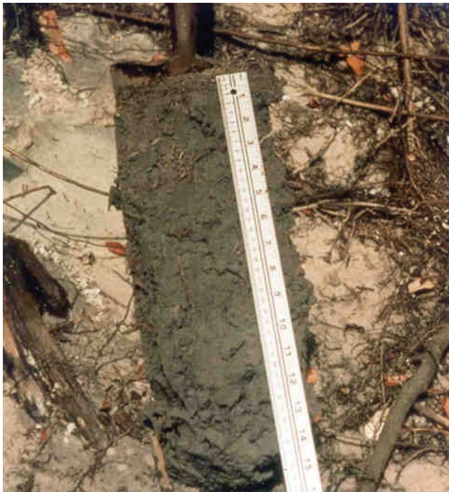
Figure 21.—Indicator S4 (Sandy Gleyed Matrix). The gleyed matrix begins at the surface of the soil.
